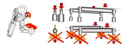
B) Planetary movements: bending rolls planetary movement that reduces frictions to minimum, frictions very common on traditional movement machines, such as diagonal or horizontal sliding guides.
