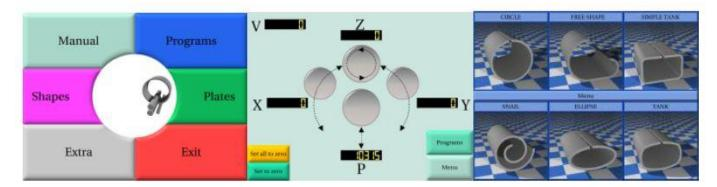
To handle a complete automatic cycle, we propose a Computerized Numeric Control called Touch Command that has been completely developed by MG Engineers. Software dedicated to our machines, instead of having the application applied to the control, as very often happens.
